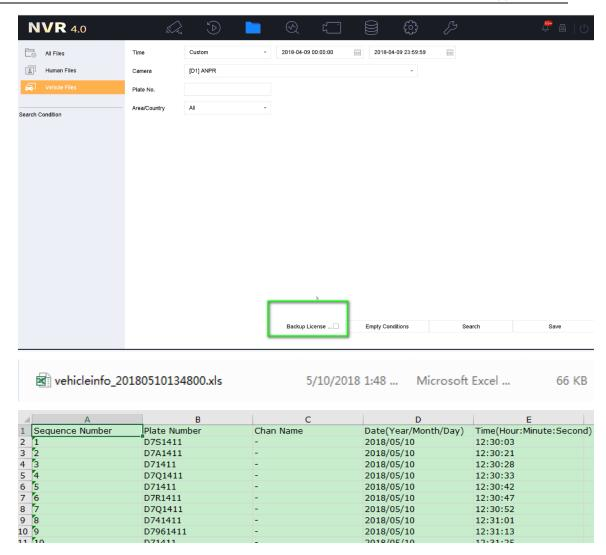
Go to Live view->Target Detection-> Select Vehicle Detection to watch the real-time captured license plate pictures & videos;
